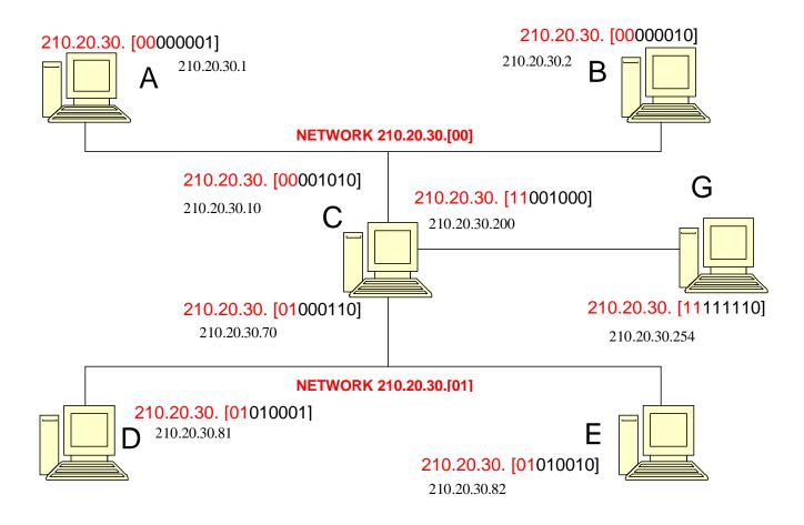
We have expanded the last byte of the IP address so that we can show the network subaddressing. The standard IP address nomenclature is shown below this expanded version.
