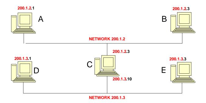
Device C is acting as a **router** between these two networks. A router is a device that chooses different paths for the network packets, based on the addressing of the IP frame it is handling. Different routes connect to different networks. The router will have more than one address as each route is part of a different network.
