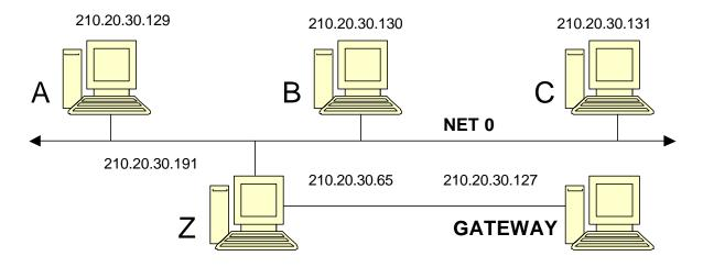
Node A is one of the many workstations on the Ethernet segment Net 0. Node Z with WANPIPE<sup>™</sup> is the gateway from this Ethernet to the Internet service provider's gateway machine G. Some of the other workstations have been labeled as B to Y for illustration, but will not be referred to in this example as their setup will be the same as for A.
